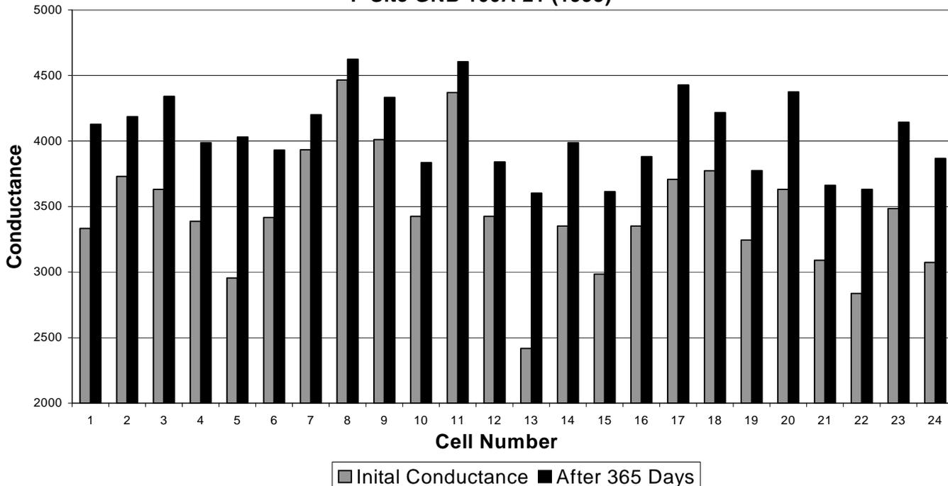
**Capacity Test Results Before & After Catalyst / Re-Hydration
