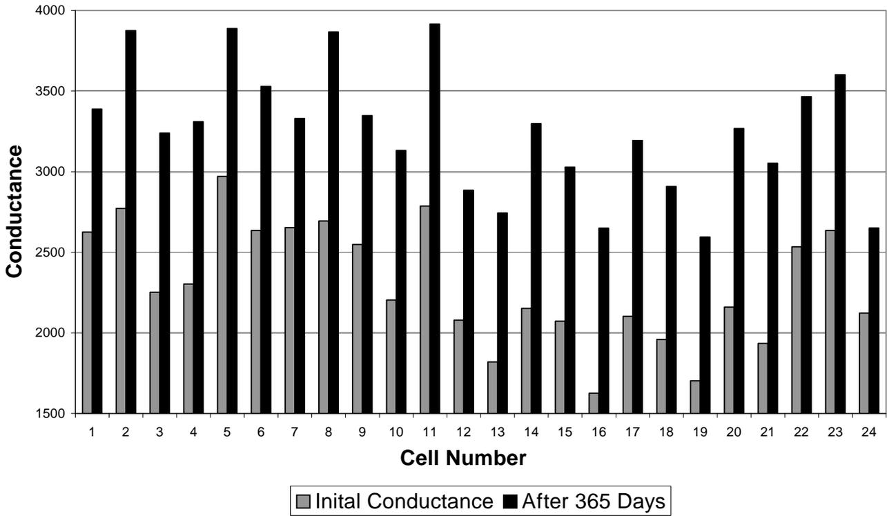
**Capacity Test Results Before & After Catalyst / Re-Hydration
